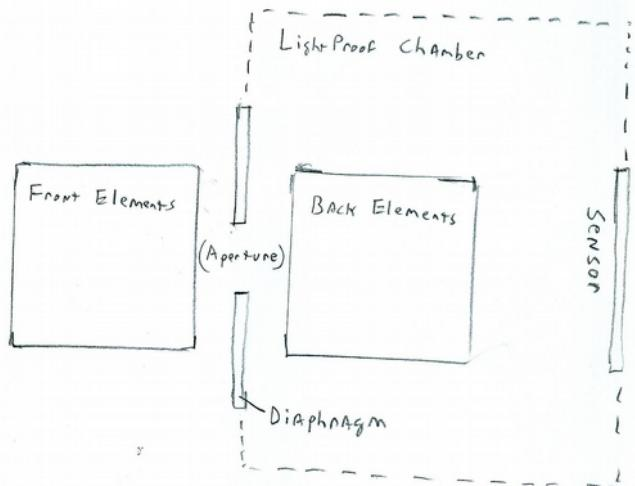
*diaphragm* - mechanical device inside a camera lens that controls the aperture
