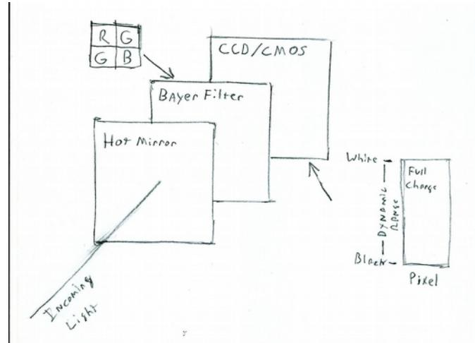
*hot mirror* - filter designed to pass visible light while blocking infrared and ultraviolet light with a sharp cutoff at either end
